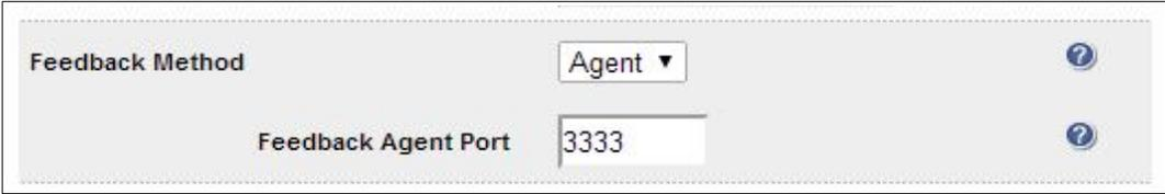
The screenshot shows a configuration panel for a Virtual Service. It contains two fields: 'Feedback Method' with a dropdown menu currently set to 'Agent', and 'Feedback Agent Port' with a text input field containing the value '3333'. Both fields have a help icon (a question mark in a circle) to their right.
