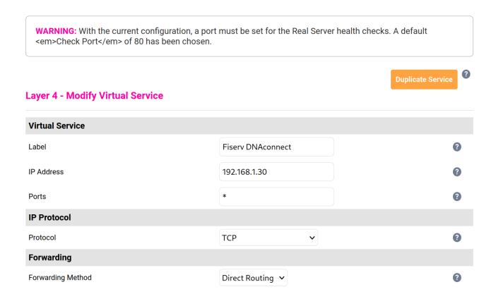
Please note the warning at the top of the WebUI. As we now use the wildcard to access the VIP, the load balancer needs to choose a port for health-checking and automatically chooses the first one, 80.
