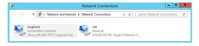
(1) Important Either adjust the commands to use the names allocated to your LAN and loopback adapters, or rename the adapters before running the commands. Names are case sensitive so make sure
