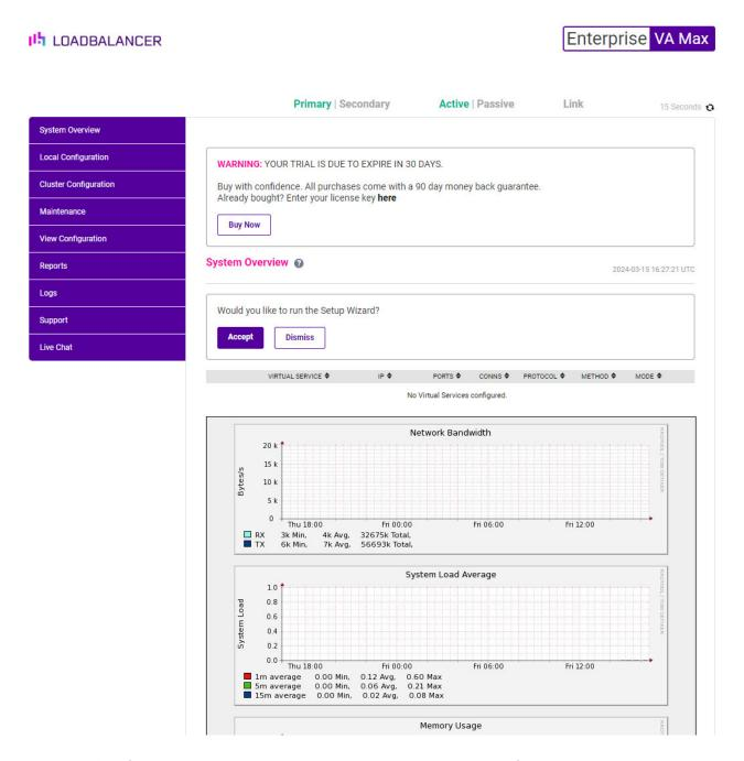
3. You'll be asked if you want to run the Setup Wizard which can be used to configure layer 7 services. Click **Dismiss** if you're following a guide or want to configure the appliance manually or click **Accept** to start the wizard.
