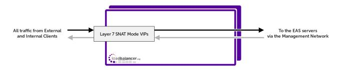
When load balancing at layer 7, performance is not as fast as the layer 4 option available in scenario 1. Layer 7 load balancing is also more intensive for the load balancer.
