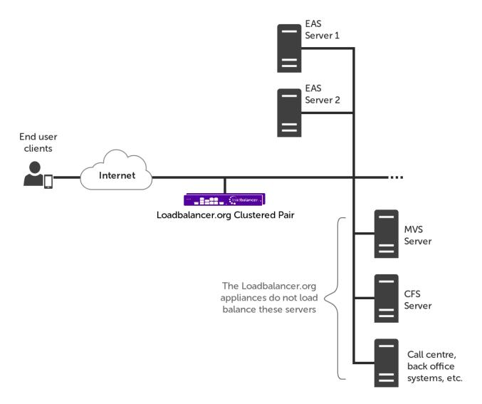
An EAS deployment can be built without a separate service network. In this case, external and internal traffic is all handled on a single internal network. All traffic must be load balanced using layer 7 SNAT mode virtual services.
