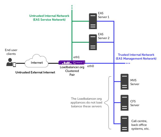
This is the recommended network configuration by Metaswitch. Two separate internal networks are used in this configuration:
