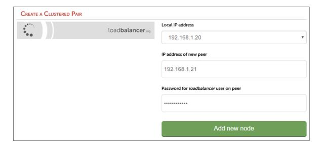
• Specify the IP address and the *loadbalancer* users password (the default is 'loadbalancer') for the slave (peer) appliance as shown above
