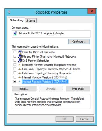
5. Ensure that Internet Protocol Version (TCP/IPv4) is selected, click Properties and configure the IP address to be the same as the Virtual Service address (VIP) with a subnet mask of 255.255.255.255, e.g. 192.168.2.20/255.255.255.255 as shown below:
