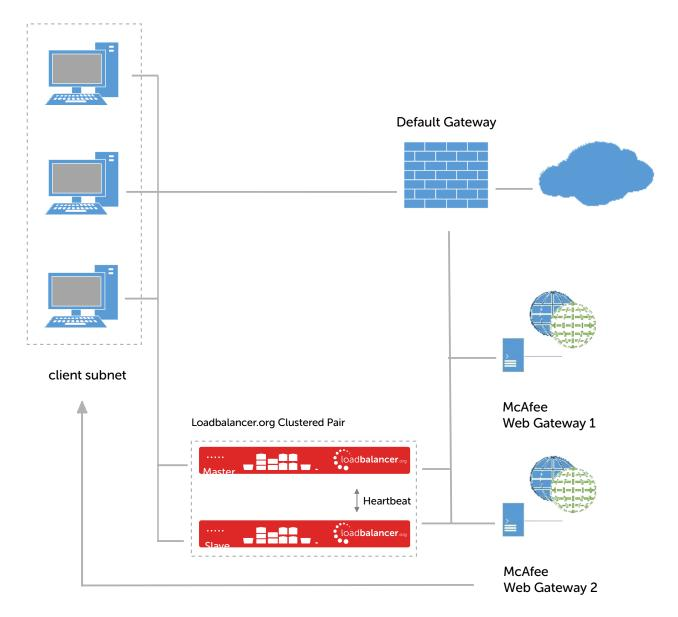
a static route is added to the Web Gateways to enable traffic to return to the client subnet via the load balancer
