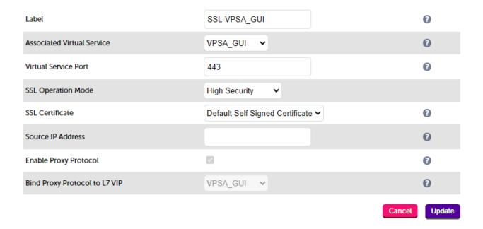
2. Set *Associated Virtual Service* to the appropriate VIP, e.g. **VPSA GUI**. This will automatically fill in the label as the VIP name with SSL inserted in front of the VIP name e.g. **SSL-VPSA GUI**.
