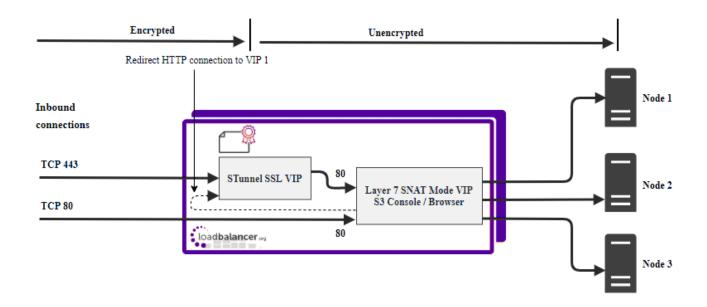
In this case, an SSL VIP utilizing stunnel is configured on the appliance and an SSL certificate is uploaded and associated to the Virtual Service. Data is encrypted from the client to the load balancer, but is un-encrypted from the load balancer to the backend servers as shown above.
