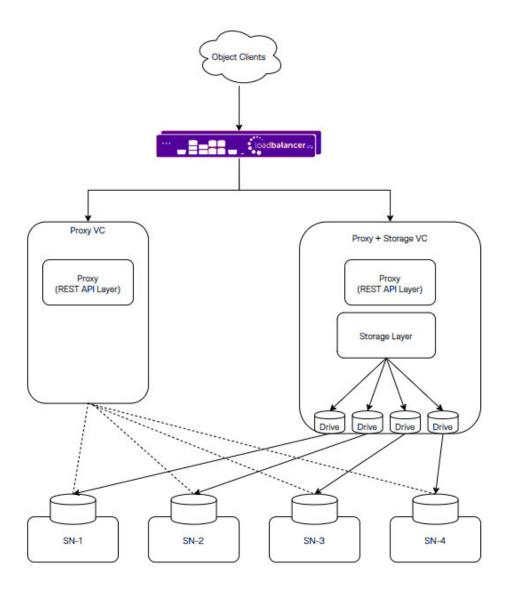
This figure shows high level logical view of VPSA Object Storage. It is a Virtual Object Store cluster, with two distinct layers:
