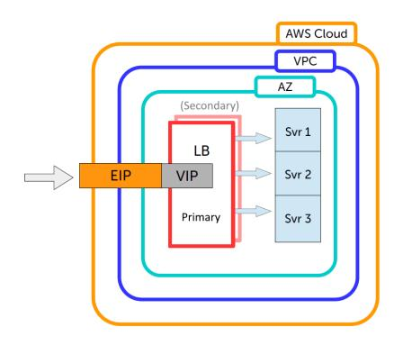
• Under normal conditions the Primary is active and the Secondary is passive. If the Primary fails, the load
