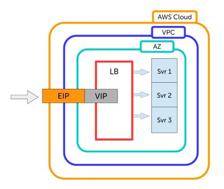
• If the load balancer instance fails for any reason, load balanced services will no longer be available.
