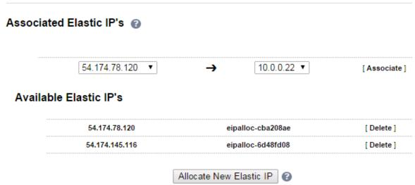
2. Under the Associated Elastic IP's section click [Associate] next to the VIPs private IP address (10.0.0.22 in this case), if no Elastic IP's are available, use the Allocate New Elastic IP button to add one.
