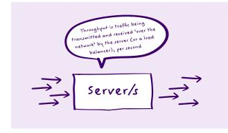
N.B. Protocol overheads mean you're only likely to actually achieve around 80% of the maximum theoretical throughput of an interface. It's also worth keeping in mind that cloud based host virtual network interface throughput may be limited by factors other than the reported speed of an interface. So while the operating system may be presented with a virtual 1Gb network interface, its actual maximum possible throughput may be far lower.
