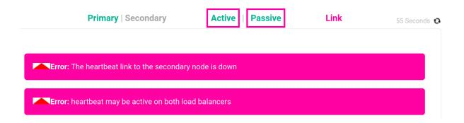
When heartbeat communication is re-established, heartbeat will automatically attempt to resolve the split brain and ensure that only one of the units is active. If heartbeat fails to do this automatically, the system status will show as follows on both units:
