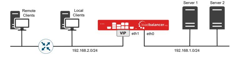
Typically ethO is used as the internal interface and eth1 is used as the external interface. This is not a requirement - each interface can be used for any purpose.
