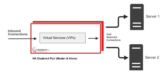
We always recommend that 2 appliances are deployed as an active/passive HA pair. The Secondary appliance automatically takes over if the Primary unit fails. For more information on configuring HA using 2 appliances please refer to Configuring HA - Adding a Secondary Appliance.
